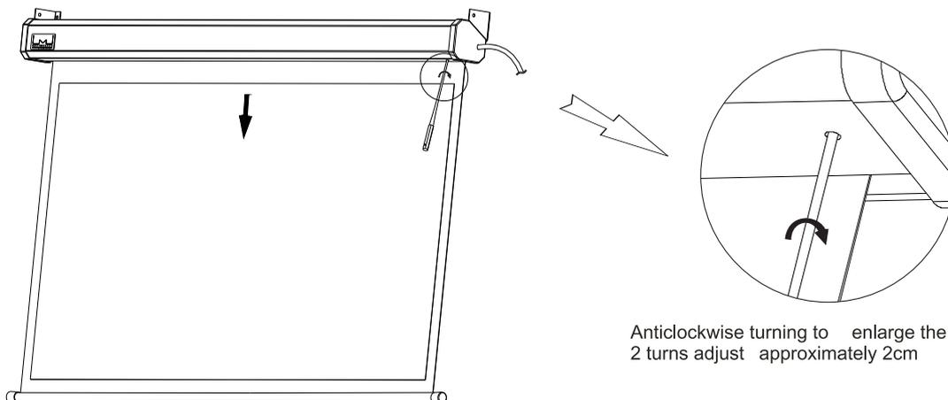
Anticlockwise turning to enlarge the top drop
